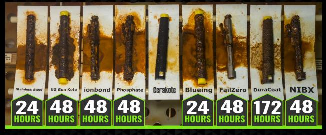
**CORROSION**HEAD TO HEAD TEST
